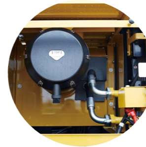
Air filter maintenance space
