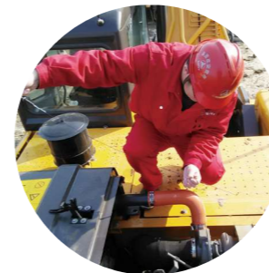
Inspect the situation of engine oil
